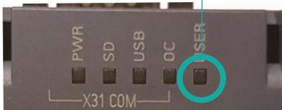
When the IoT reboots the red "USER" led is powered off and the setup procedure is successful.
