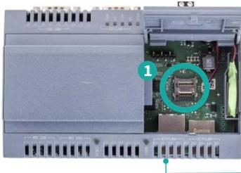
1 Insert microSD card in the slot by lifting the front panel
